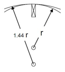
Figure 1. The two arcs of circles are shown representing the bend of floor sheathing from gravity loads. The gravity loading is assumed to be equal; however, the stiffness varies by 44%. The curvature is exaggerated for illustration purposes.
