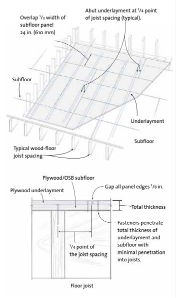
are more conservative than specified in ANSI A108-1999, Section AN-3.4.1.3, which states, "locate nails at 6-inch centers along panel edges and 8-inch centers each way throughout the panel." Closer nail spacing as given in Table 1 on p. 198 will better guard against voids between
