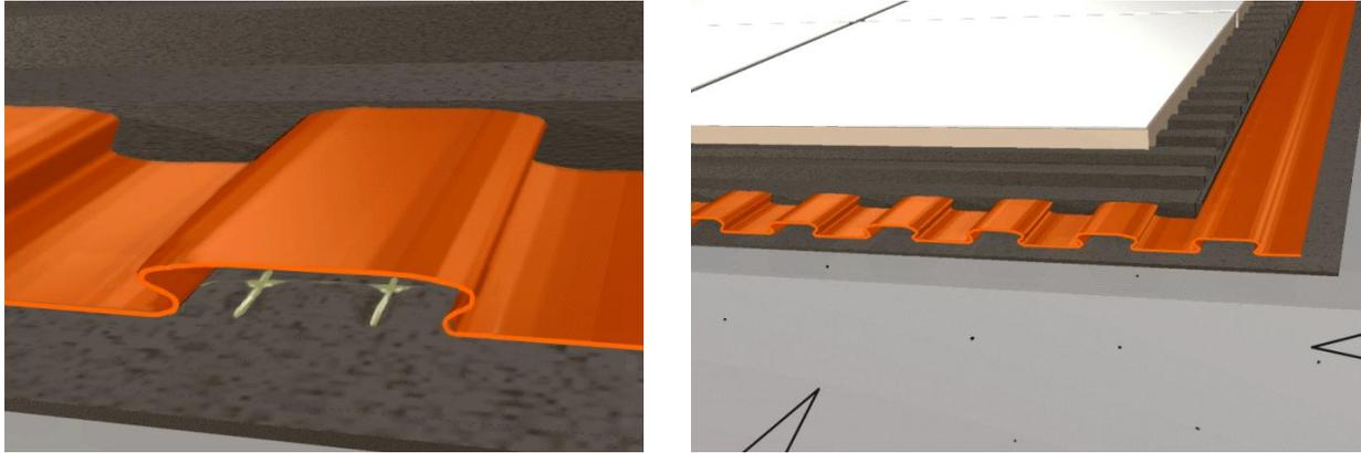
Figure 4. The modern analog to the sand strata method commercially known as: DITRA. The image on the left illustrates the corrugated nature of the polyethylene sheet, with the polyethylene webbing bonded to the bottom. The right shows DITRA in a typical installation, serving to de-couple the substrate from the tile layer, allowing the tile assembly to act independently from the substrate.
