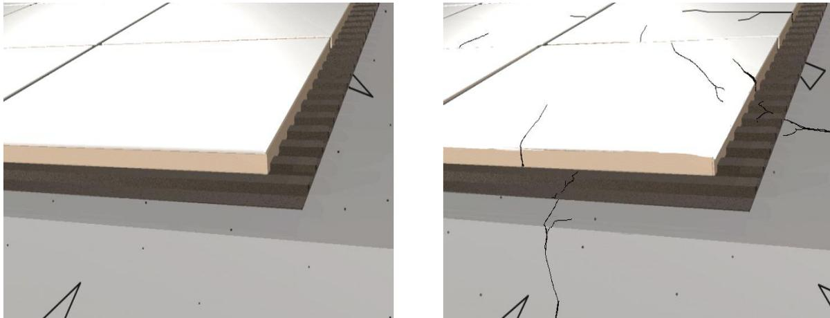
Figure 3. The direct bond method of tile installation, in which the tile is directly bonded to the substrate using a thin bond coat. No method of de-coupling is used in this case and, as illustrated on the right, cracks in the substrate become cracks in the tile.
