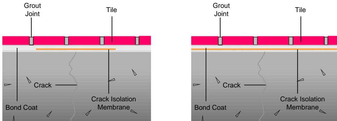
Figure 6. Schematic illustration of the two common approaches used with crack isolation membranes. The diagram on the left shows the membrane used to directly address existing cracks in the substrate. The illustration on the right uses the crack isolation membrane over the entire substrate surface. The use of these membranes does not eliminate the force conductive bonding situation, which leads to cracking in the tile assembly due to strain transfer from the substrate.
