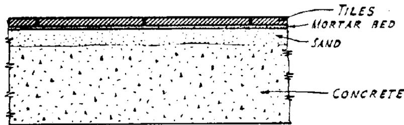
Figure 1. A schematic cross-section of the traditional method for de-coupling the tile from the substrate – the sand strata method.
