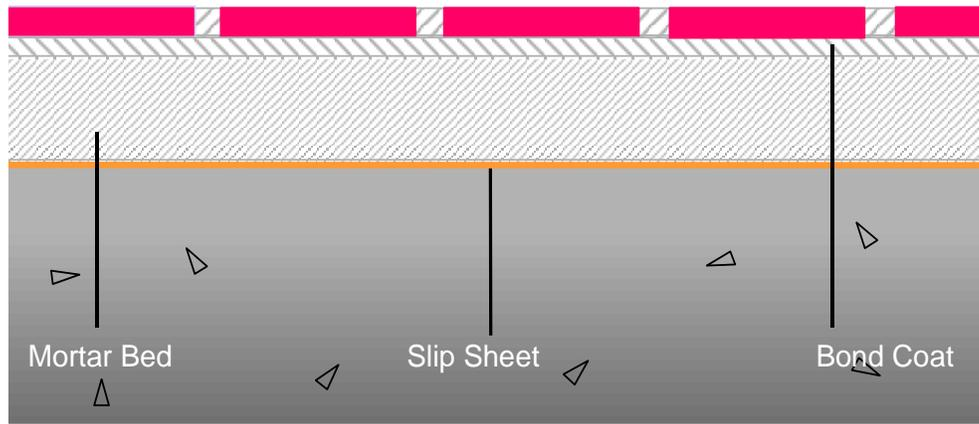
Figure 2. The more recent approach to the sand strata method—the wire-reinforced two-inch mortar bed over a slip sheet (cleavage membrane). The wire has been omitted for clarity.
